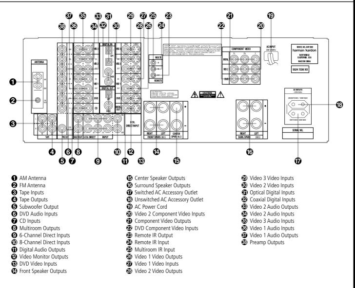
**NOTE:** To assist in making the correct connections for multichannel input/output and speaker connections, all connection jacks and terminals have been color coded in conformance with the latest CEA standards as follows:
